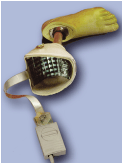
Figure 1. Sensors inserted in socket.
